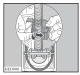
With the supplied spanner unscrew and remove the central rear bolt A. Slide out the relevant plastic spacer.
